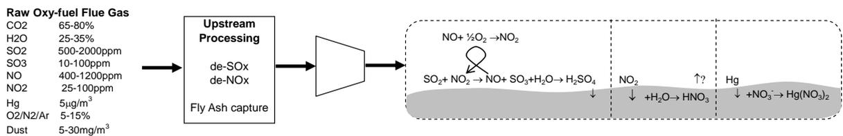
**Figure 8.** Interaction of NO<sub>x</sub>, SO<sub>x</sub> and Hg during compression of oxy-fuel flue gas
