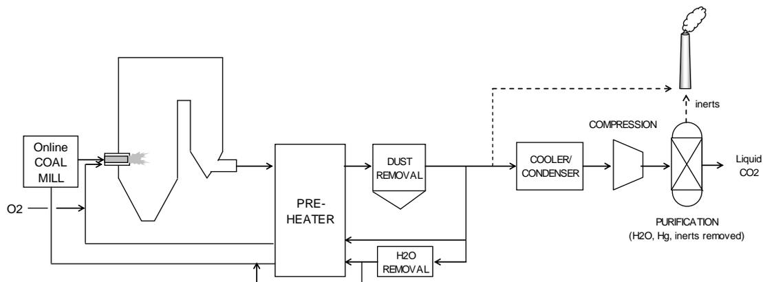
**Figure 5.** Diagram of the Callide Oxyfuel Project
