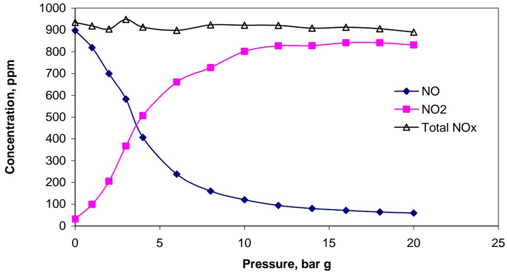
**Figure 12.** Effect of pressure on the oxidation of NO to NO<sub>2</sub> (in 4% O<sub>2</sub>) without water. The points in this figure and Figures 13 to 16 correspond to results for individual experiments at a number of pressures for common periods of 10 minutes.
