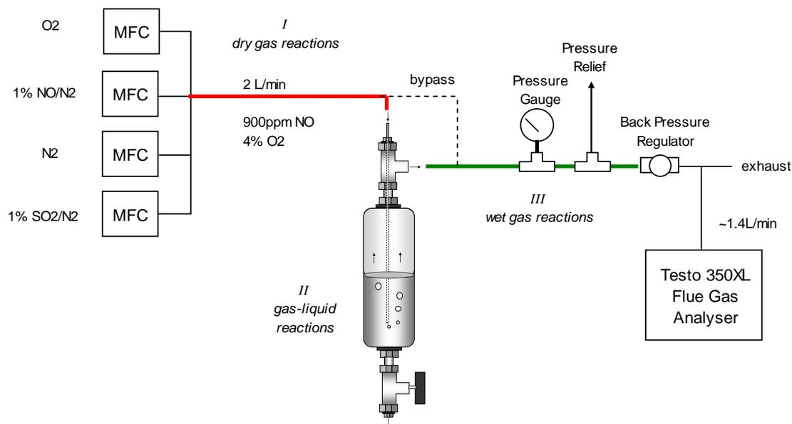
**Figure 11.** Pressurised laboratory apparatus for contacting  $\text{NO}_x$  gases with water, indicating the three different conditions for reactions involving I - dry gas, II – gas-liquid and III – wet gas
