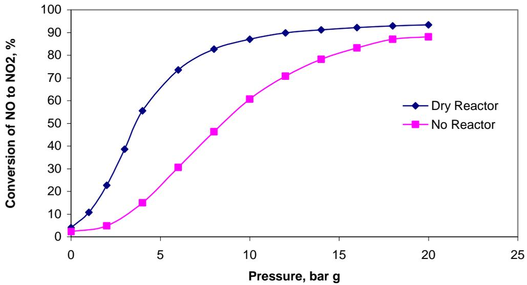
**Figure 13.** Comparison of NO<sub>x</sub> conversion in reactor and transport lines showing effect of residence time
