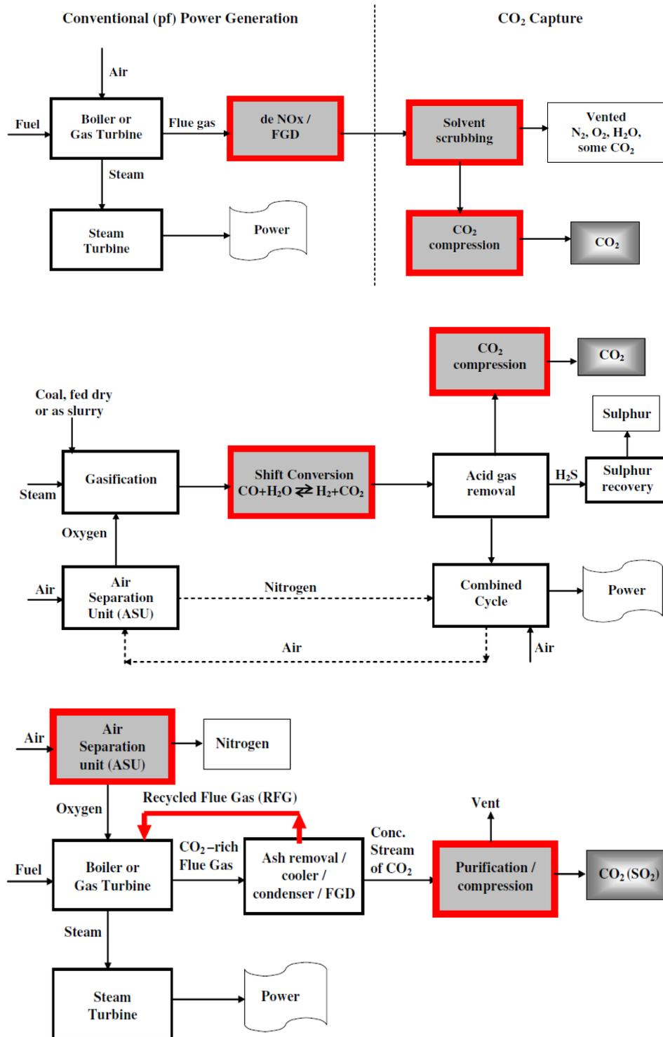
**Figure 3.** Main technologies for CO<sub>2</sub> capture from coal fired electricity generators; post combustion capture (top), Integrated Gasification & Combined Cycle-CCS (middle) and oxy-fuel combustion (bottom).
