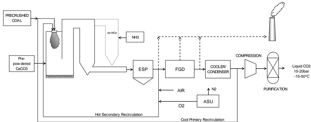
**Figure 6.** Diagram of Vattenfall's Schwarze Pumpe Oxyfuel pilot plant
