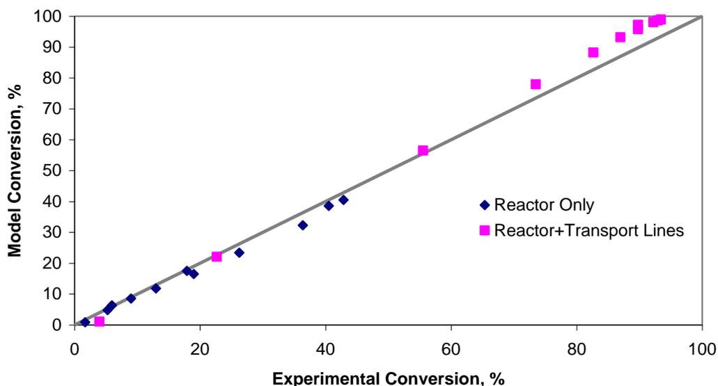
**Figure 14.** Evaluation of global kinetic model detailed in the Appendix to measured experimental results, with results for two differing durations corresponding to residence times in the reactor only, and the reactor with transport lines
