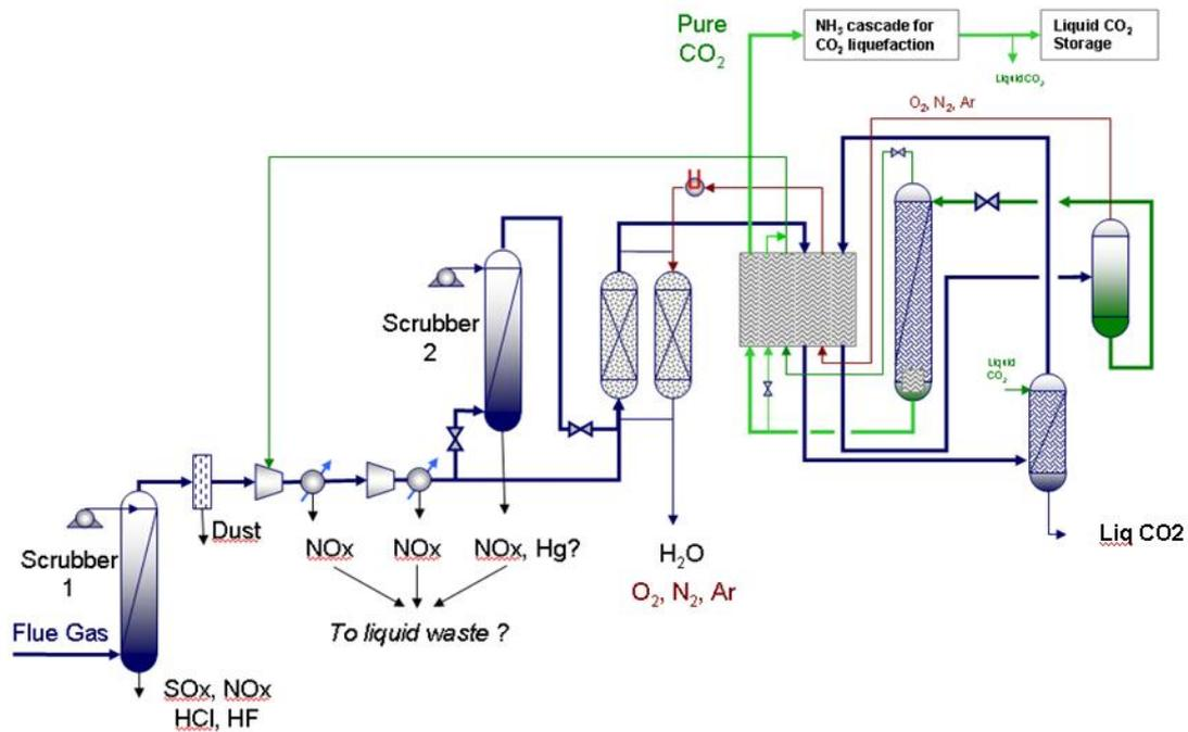
**Figure 8.** Callide Oxy-fuel compression circuit, from [13]
