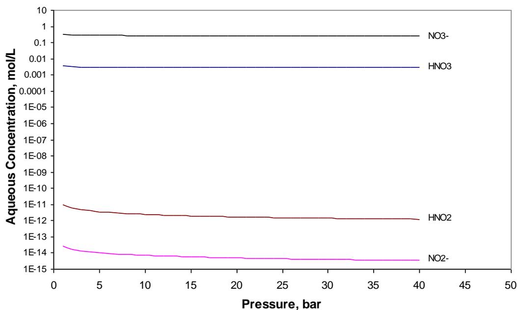
**Figure 20.** Thermodynamic modelling of aqueous species in wet NO<sub>x</sub> system using FACTSage at 25°C (1000ppm NO, 20% H<sub>2</sub>O, 3% O<sub>2</sub> starting)
