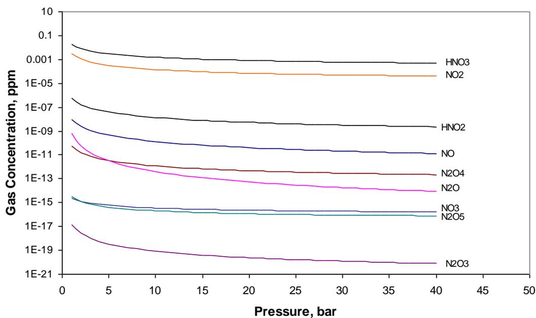
**Figure 19.** Thermodynamic modelling of gas species in wet NO<sub>x</sub> system using FACTSage at 25°C (1000ppm, NO, 20% H<sub>2</sub>O, 3% O<sub>2</sub>, balance CO<sub>2</sub> starting)
