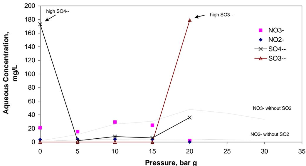
**Figure 17.** Aqueous  $\text{NO}_x$  and  $\text{SO}_x$  species present in solution after 10 minutes contact time (feed gas mix 1000ppm  $\text{SO}_2$ , 1000ppm  $\text{NO}$ , 3.5%  $\text{O}_2$ ,  $\text{N}_2$  balance). Lines marked in grey are results for  $\text{NO}_x$  only contacting.
