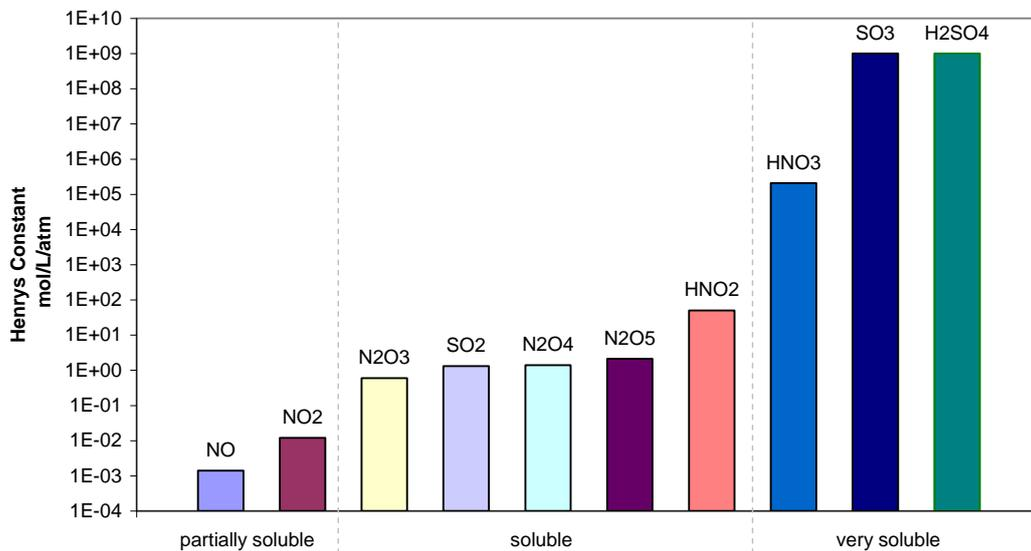
**Figure 10.** Comparison of solubilities of  $\text{NO}_x$  and  $\text{SO}_x$  gaseous species in water using Henry's Constant at 25°C (logarithmic plot, showing orders of magnitude differences). Note that  $\text{SO}_3$  and  $\text{H}_2\text{SO}_4$  values are given as infinite in [20] but expressed here as a value.
