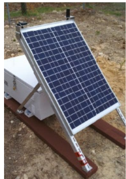
The seismic stations are relatively small and self-powered. Recorded data will be transmitted to UWA remotely using the mobile 3G/4G network.
