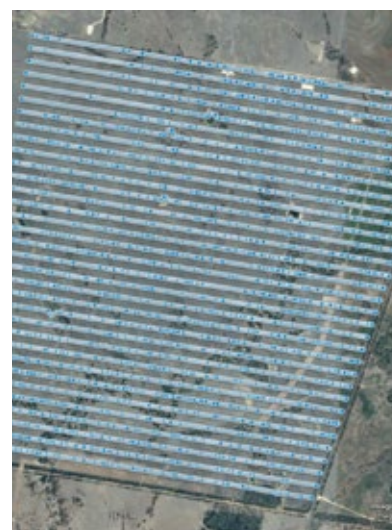
Array of 10,055 1-C stations of passive seismic survey in Glenhaven
