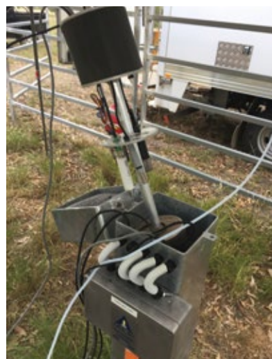
One of CTSCo's monitoring stations comprising two soil vapor wells and two groundwater wells (top). Instruments are deployed downhole within a packer system and provide real-time data acquisition (bottom)
