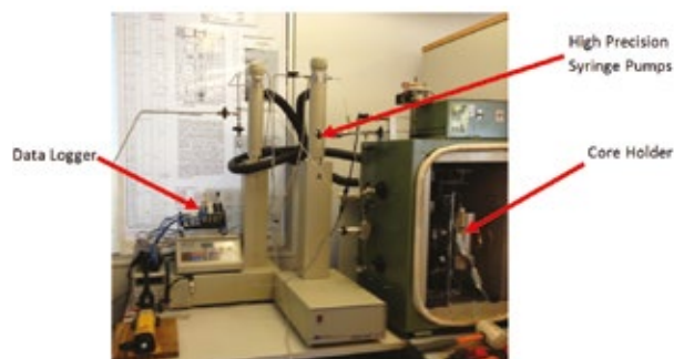
Apparatus for capillary pressure measurements at reservoir conditions.
